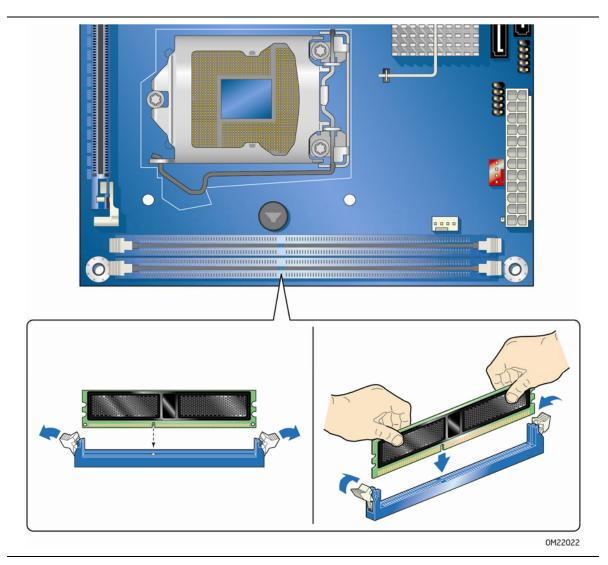
Figure 16. Installing a DIMM
